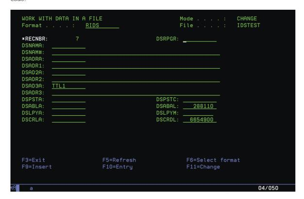
Note that the TTL1 has been placed in the DSAD3A field. This is an attribute field which has the DDS TEXT keyword that contains 'Atr Excel Fld'. (See the previous example for a full explanation of the usage of the DDS keyword TEXT)
