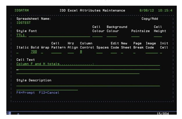
Here is a style called TTL1 which has the bold set on and the column control value set to 'N'. The column control being set to 'N' tells the system not to adjust the column width to allow for the width of the data.
