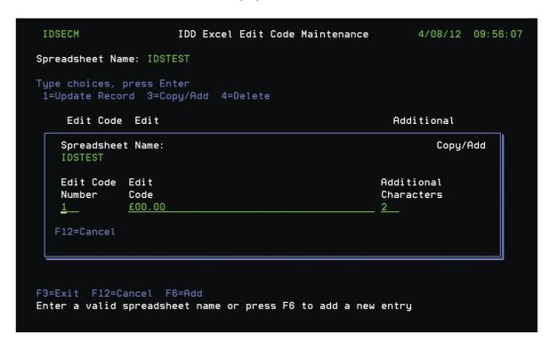
The above code tells the system that when the edit code 1 is applied to data that there should always be 2 decimal places and be preceded by a  $^{\prime}$ £ $^{\prime}$  sign. Press enter to create the edit code 1.
