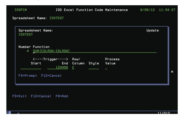
Note that the function now contains the constant 'COL'. When the trigger value of 123456 is found the 'COL' constant will be replaced with the column that is currently being processed.
